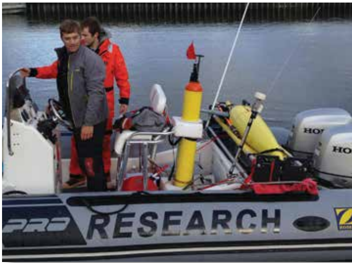
Acoustic Seaglider and QUEphone deployment off Washington. Two instruments were deployed from the 21-ft RHIB.
