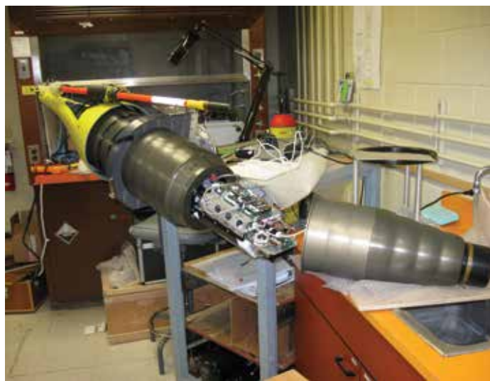
The PAM board installed in the Kongsberg Seaglider.
