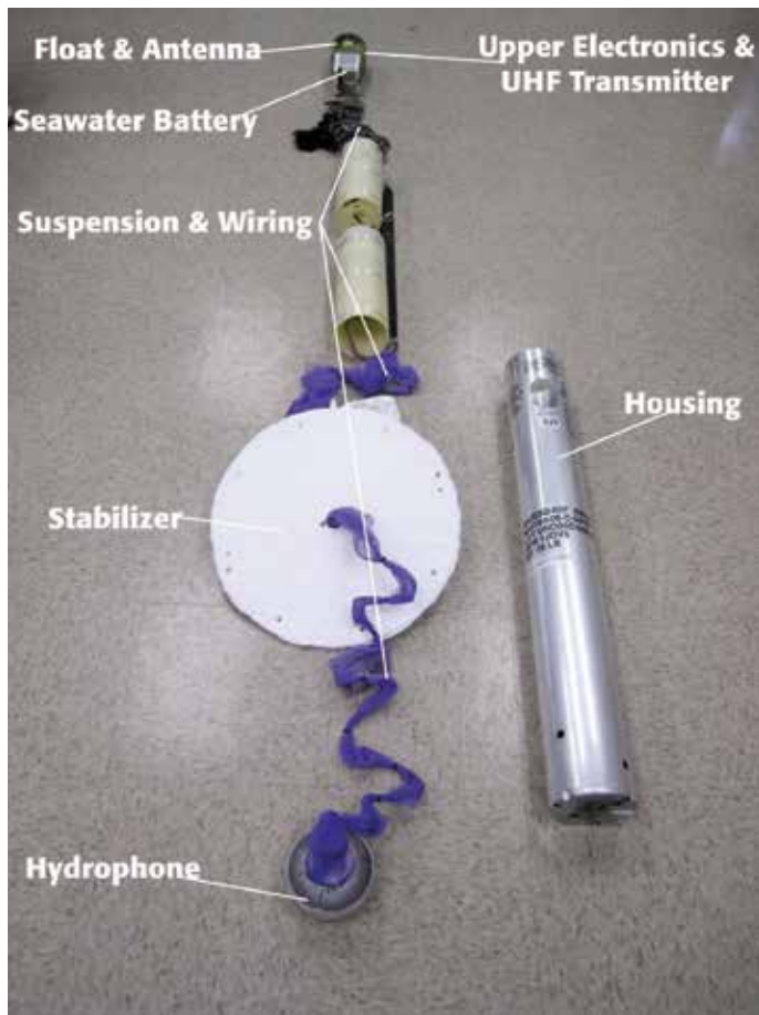
Parts of a SSQ-Q53F sonobuoy after being removed from its housing.
